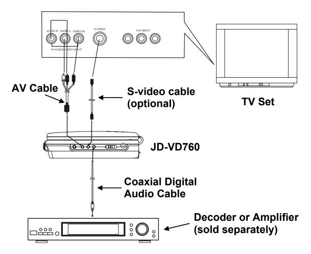
Once the JD-VD760 and all other appliances are securely connected, plug all units into AC wall outlets and switch the power on.
